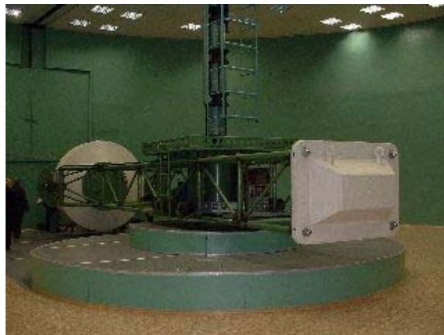
Fig. 51: One-person rated centrifuge of the GCTC Gagarin Cosmonauts’ Training Centre
