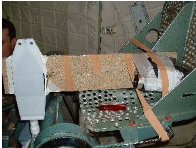
Fig. 53: Lung model with video camera for verification of the lung excursion placed inside the centrifuge
