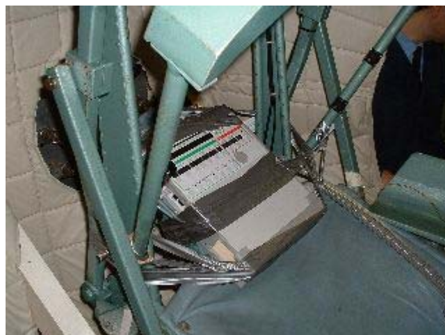
Fig. 52: Fixation of the ventilator to the centrifuge seat
